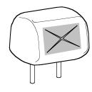
Using a sharp, adjustable-depth blade knife, make a diagonal cut beginning 1/4" INSIDE from one corner, and ending 1/4" INSIDE from the opposite corner.
