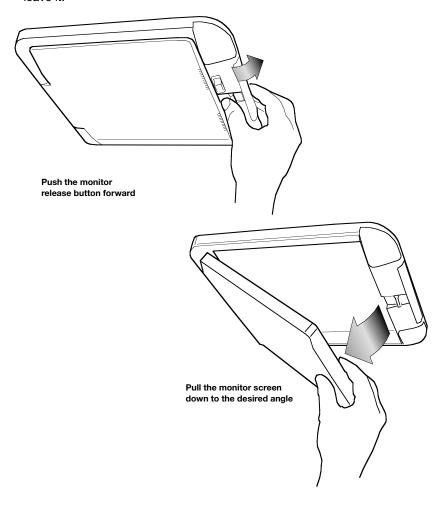
To avoid accidental damage, we suggest you always close the monitor assembly when it is not in use. To do so, rotate the monitor back to a 0° left-to-right position, and push it up into the monitor base until you hear a "click." Test that it is secured by gently pulling down on monitor frame.
