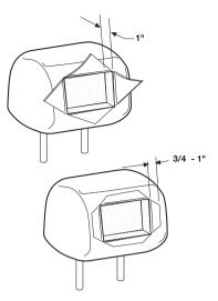
Set the adjustable blade to 1" depth, and cut around the edges of the hole, staying 1/4" inside the edge. Pull up one corner of the foam rectangle, and use the blade to cut underneath – remove a small section at a time, using the "pull up and cut" method for uniform depth. If necessary, use a Dremel tool or other appropriate tool to remove any other obstructions present.
