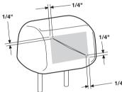
Using a sharp, adjustable-depth blade knife, make a diagonal cut beginning 1/4" INSIDE from one corner, and ending 1/4" INSIDE from the opposite corner.
