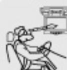
Installation of all TV monitors must be out of the driver's field of vision.
