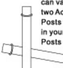
Since the spacing of the mounting holes can vary on different vehicles we supply two Adapter Posts. Use these Adapter Posts when the headrest mounting holes in your seat are too large for the Adapter Posts of the headrest monitor.
