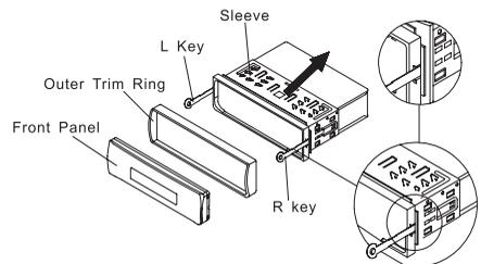
6. Mount the sleeve by inserting the sleeve into the opening of the dashboard and bend open the tabs located around the sleeve with a screwdriver. Not all tabs will be able to make contact, so examine which ones will be most effective. Bend open the appropriate tabs behind the dashboard to secure the sleeve in place.
