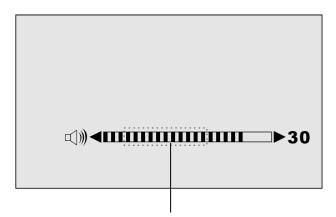
Playback of audio which comes into the player via the front panel AUX IN jack has limited settings available for adjustment. Press the center area of this scale to select the following audio adjustment settings menus: VOLUME > BASS > TREBLE >
