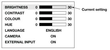
To adjust a setting, simply touch the on-screen button for that setting. After it is selected, use the VOL-/+buttons to change the setting. You can also press the button on the display to adjust it.
