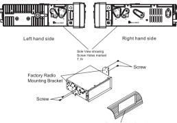
Fasten the unit to the factory radio mounting brackets. Align the screw holes on the bracket with the screw holes on the unit, and then tighten the screws (5x5mm) on each side. Note: The outer trim ring, sleeve and the metal strap are not used for method B installation.
