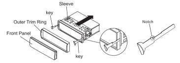
6. Mount the sleeve by inserting it into the opening of the dashboard and bend open the tabs located around the sleeve with a screwdriver. Not all tabs will be able to make contact, so examine the opening to determine which tabs will be most effective. Bend open the appropriate tabs behind the dashboard to secure the sleeve in place.
