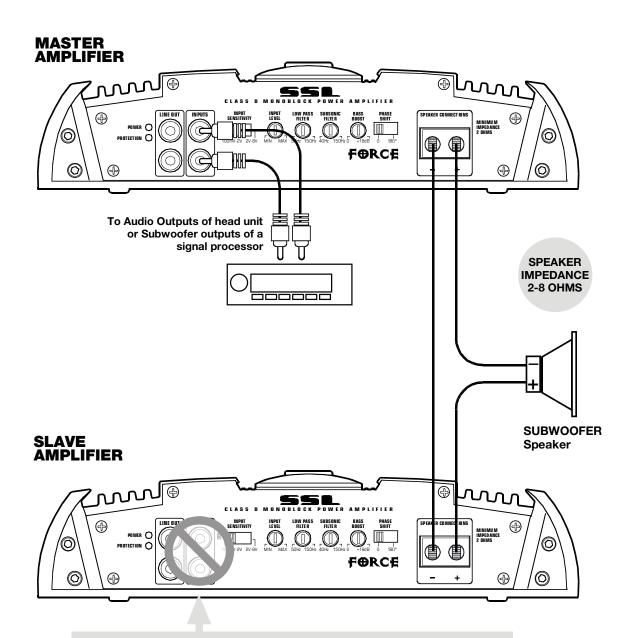
PLEASE NOTE: In this MASTER AMP/SLAVE AMP configuration, the Slave amp receives its audio signal from the Master Amp. Therefore, DO NOT USE THE INPUTS ON THE SLAVE AMP!)
