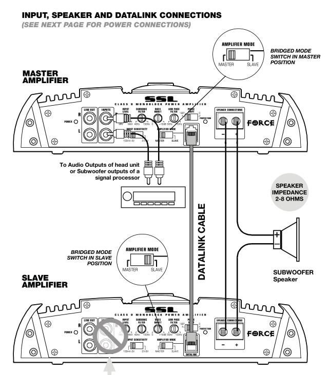
PLEASE NOTE: In this MASTER AMP/SLAVE AMP configuration, the Slave amp receives its audio signal from the Master Amp. Therefore, DO NOT USE THE INPUTS ON THE SLAVE AMP!)
