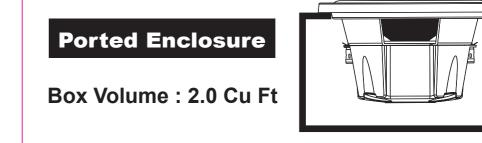
Box is given as internal air volume including driver displacement
